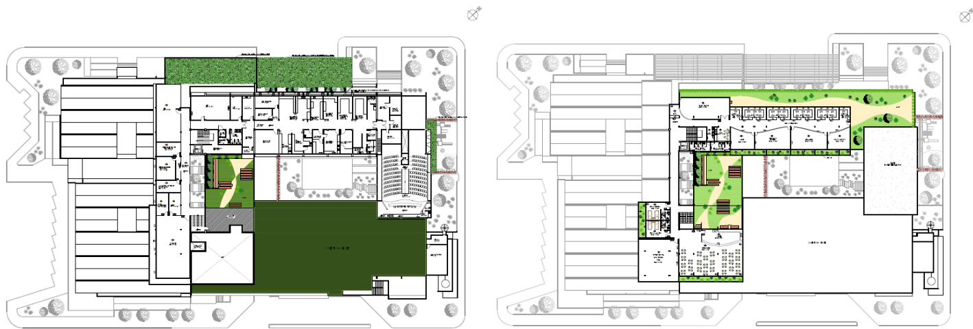
Figure 3 (a) Floor plan of the second level and (b) floor plan of the third level of HemoCE blood center.
